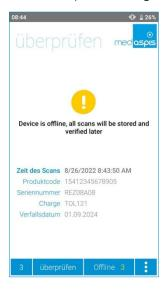
Nevertheless, the FMD Speed Scanner remains operational. Data is recorded, work does not have to be interrupted. All codes captured during the offline phase are saved in the handheld device itself; under no circumstances data records are lost. The number of codes captured in this phase is shown in yellow in the bottom bar.
