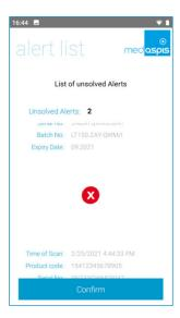
In this case, the scanner is stopped, you can no longer scan, you have to take care of the alert. This process is documented by clicking the "Confirm" button on the Speed Scanner display. Analogously, this is noted in the Scan History.
